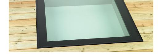
Manufactured from our extruded aluminium profile which is thermally broken with two polyamide insulating sections and factory glazed with a walk-on specification insulating glass unit. The latest regulations for thermal performance and safety have been surpassed by the ODC Walk-on Rooflight.
