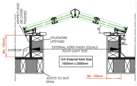
Example above shows a Gabled  $1500 \times 2000$  style. Note: The size you order is the FINISHED EXTERNAL kerb size to build.
